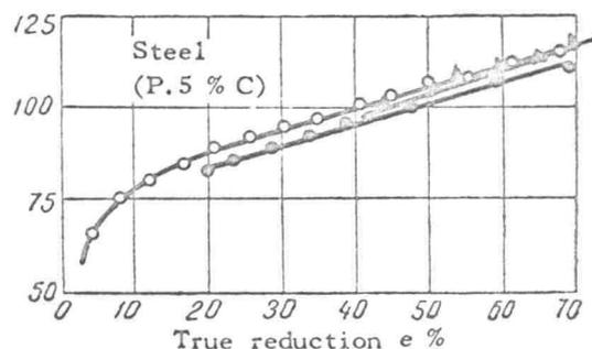
Fig. 1. Tensile test diagrams for St.50 specimens
